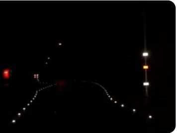
Armorstud's 360° unidirectional optical reflex technology reflects light back to its projected source from any area with in its 360 degree radius. Armorstud's optical reflection characteristics provide winding roads and turns a distinct visible marking system for all oncoming motorists.
